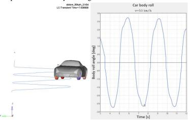
Fig. 5. Vehicle body roll analysis in MotionView software
