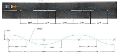
Fig. 1. Slalom trajectory curve of the tested vehicle
