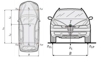
Fig. 2. Wheel forces acting on the vehicle – top view (left) and axle load (right)
