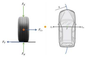
Fig. 4. Considered forces acting on the wheel (left) and forces acting on the vehicle during slalom traversing (right)
