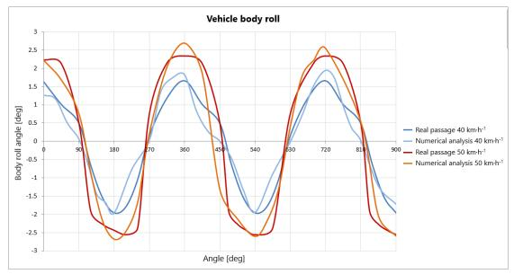
Fig. 8. Graph of body roll depending on vehicle position
