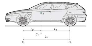
Fig. 3. Wheel forces acting on the vehicle - side view
