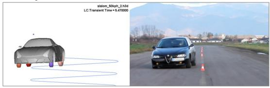
Fig. 7. Comparison of simulation with real vehicle passage
